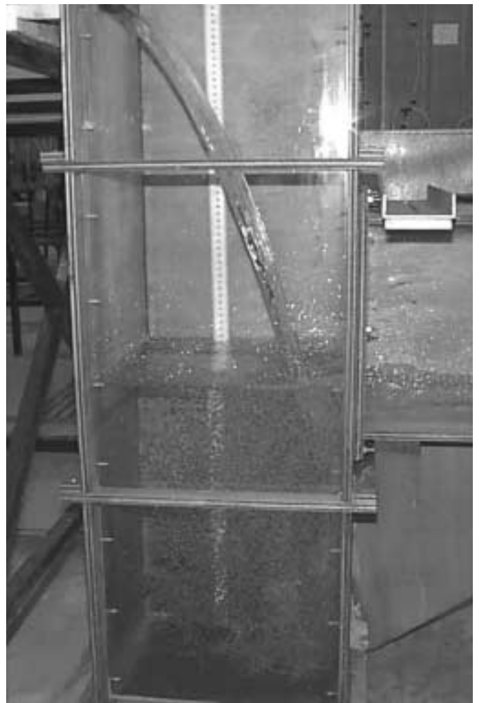
Fig. 3 Photographs of the physical models. (A) Photograph of the model 1 (Regime R1, Q = 0.001 \text{ m}^3/\text{s} ) (high-speed photograph)
