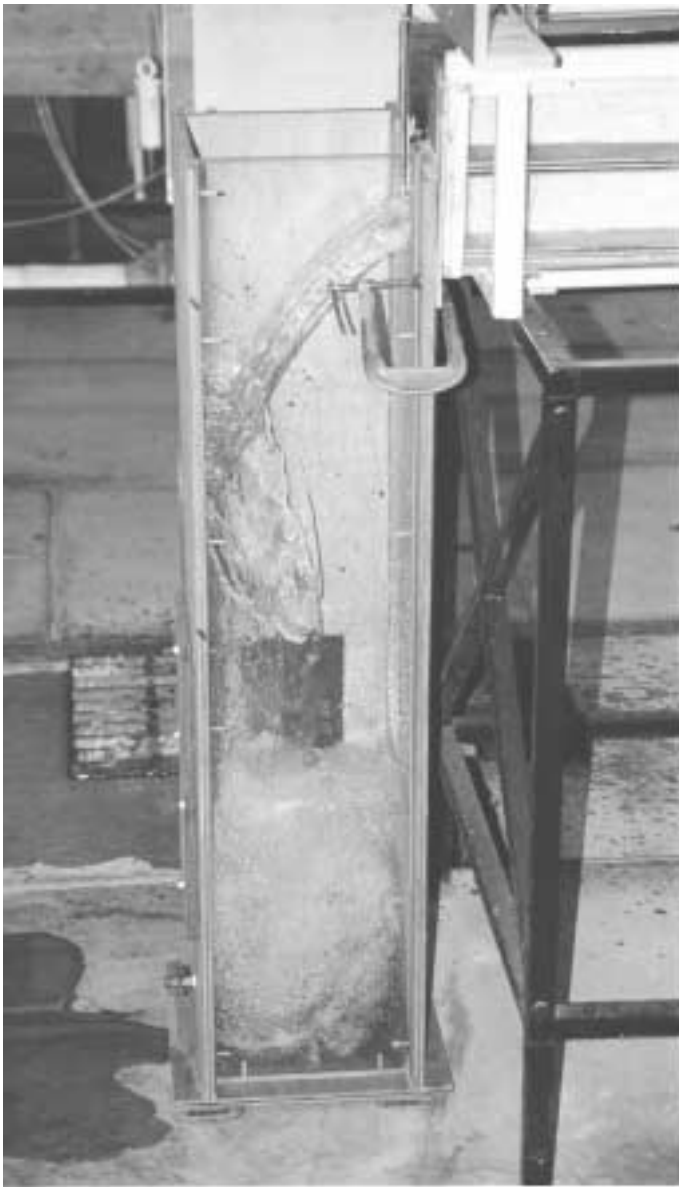
Fig. 3 Photographs of the physical models. (B) Photograph of the model 3 (Regime R3, Q = 0.004 \text{ m}^3/\text{s} )
