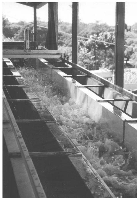
Fig. 2. High-shutter-speed photograph, looking upstream for d_c/h = 1.86 , highlighting the rapid onset of self-aeration for free-surface aeration down a very flat stepped channel [ \theta = 3.4^\circ , q = 0.15 m 2 /s, h = 0.0715 m (Chanson and Toombes 2002)]
