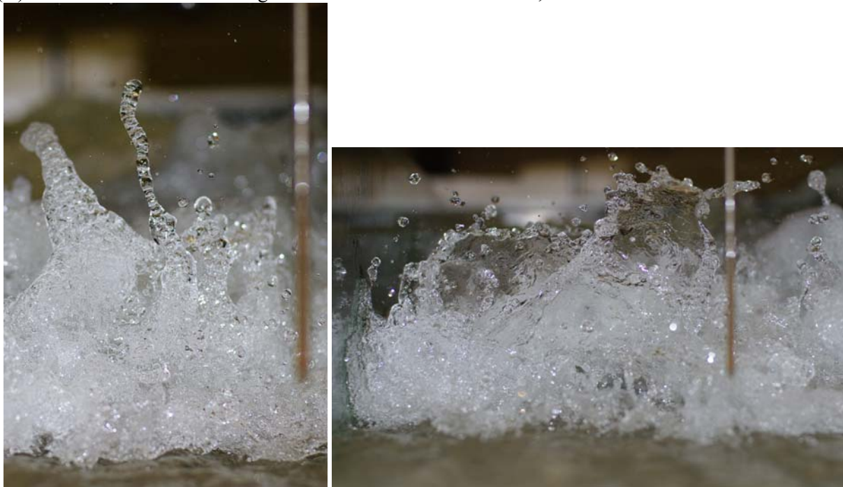
(B) Air-water projections in hydraulic jumps, looking downstream at the impingement point and free-
