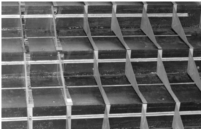
Figure 3. Photograph of the stepped invert with 7 vanes (Configuration 3).
