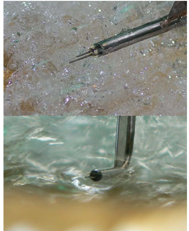
Figure 6: Photograph of the dual-tip conductivity probe ( \varnothing = 0.25 mm). Top: Three-quarter view, flow from bottom left to top right, Re = 3.5 \times 10^5 . Bottom: Looking downstream at the probe tip, d_c/h = 1.59 , Re = 7.9 \times 10^5 .
