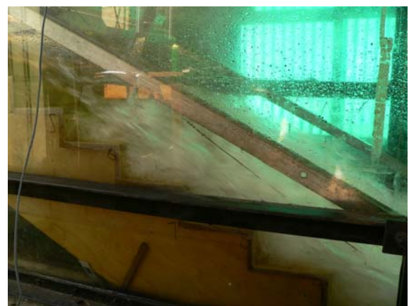
(A) d_c/h = 1.15 , Re = 4.85 \times 10^5 , inception of free-surface aeration at step edge 4
