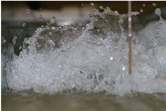
(B) d_1 = 0.0395 m, x_1 = 1.5 m, Fr_1 = 5.1 , Re = 1.3 \times 10^5 - Shutter: 1/180 s at f/2.5 , ISO 100
