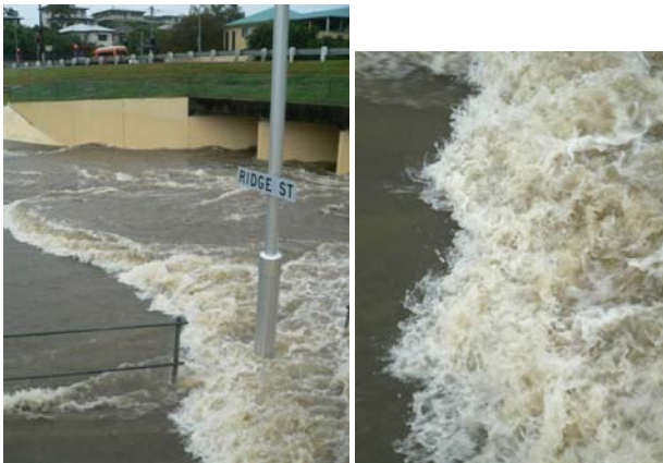
Figure 1. Hydraulic jump in a culvert inlet and details of the roller free-surface - Re \sim 3 \times 10^6 , Shutter speed: 1/80s, Flow from left to right.
