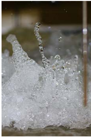
(A) d_1 = 0.0395 m, x_1 = 1.50 m, Fr_1 = 5.1 , Re = 1.2 \times 10^5 - Shutter: 1/180 s at f/2.5 , ISO 100
