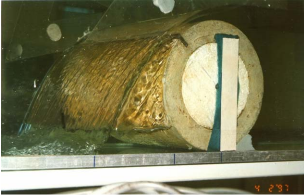
(A) Flow from right to left : q = 0.0048 \text{ m}^2/\text{s} , d_1 = 0.178 \text{ m} , R = 0.117 \text{ m} , \phi_{\text{def}} = 45 \text{ deg.} , h = 0.004 \text{ m}
