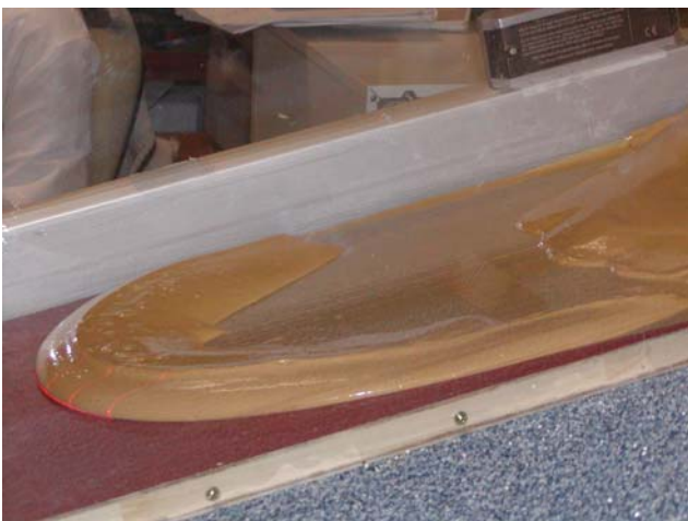
(C) Flow type III, Test 08, C_m = 0.15 , rest period: T_o = 2400 s - Sideview of the head packet
