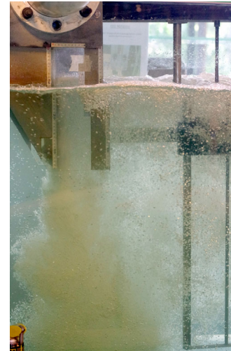
Figure 1. Air entrainment at a vertical supported jet. Flow conditions: V_1 = 4.5 m/s, d_1 = 0.0114 m, Fr_1 = 13.5 , Re_1 = 5.14 \times 10^4 .
