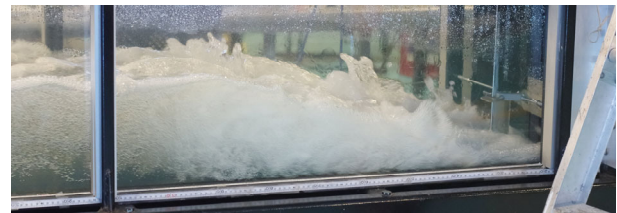
Figure 2. Air entrainment at a horizontal supported jet or hydraulic jump. Flow conditions: V_1 = 4.5 m/s, d_1 = 0.0112 m, Fr_1 = 13.5 , Re_1 = 5.14 \times 10^4 .
