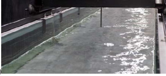
Figure 1. Standard box culvert modelling. (a) Prototype box culvert inlet beneath Paradise Road, Logan QLD. (b) Complete box culvert model ( B = 0.15 m). (c) Culvert barrel model (barrel width B = 0.5 m).
