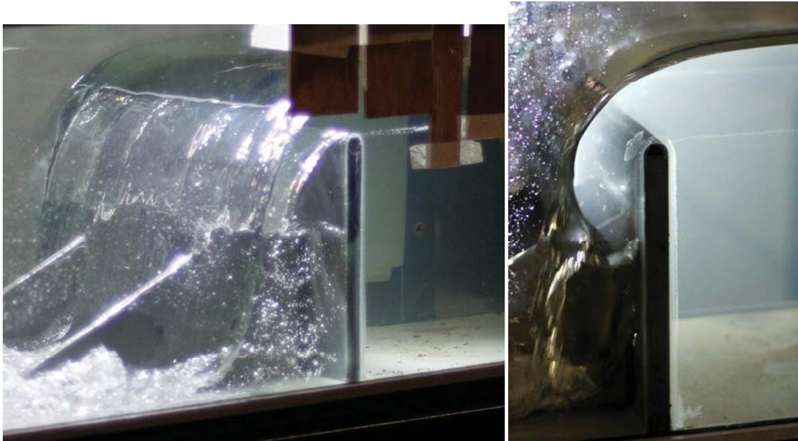
Figure 2. Overflow experiments on half-round circular weir with flow direction from right to left. Left: detached nappe for q = 0.0426 \text{ m}^2/\text{s} , (H-P)/r = 7.19 ; Right: attached nappe for q = 0.0554 \text{ m}^2/\text{s} , (H-P)/r = 7.94 .
