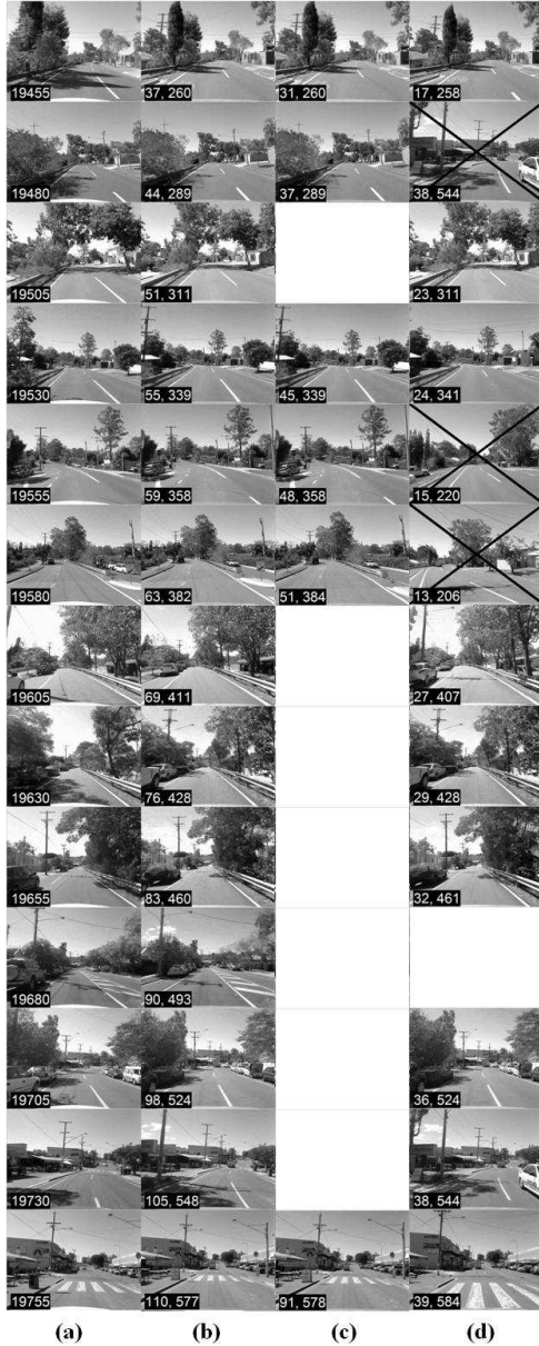
Figure 17 – (a) A sequence of frames from the second dataset, numbers indicate the frame number (b) Recalled visual templates with visual expectation, T_D = 0.045 , P = 97.0\% , R = 78.7\% . Numbers are in the format (template number, associated frame number). Blank frames indicate false negatives, crossed frames indicate false positives. (c) Recalled templates without visual expectation for a matching precision level. (d) Recalled templates without visual expectation for a matching recall level.
