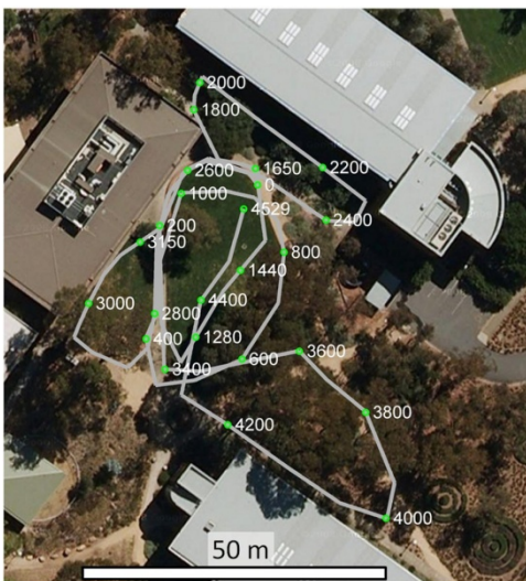
Fig. 5. The robot trajectory through the environment, projected onto a 2D terrain photo (© Google Maps). The order of traversal is indicated by the frame number labels.
