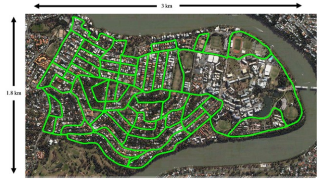
Figure 2 – St Lucia test environment, consisting of a 66km road network covering approximately 6 square kilometres. Image © IEEE Transactions on Robotics 2008.
