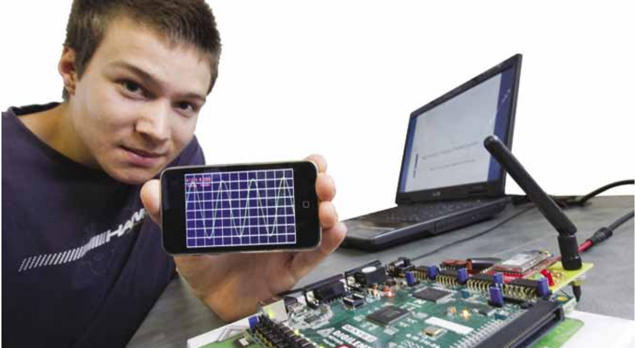
Mechatronic Engineering student Craig Haywood examined the capabilities of the modern smart-phone as an engineering display platform through the design and implementation of a portable digital oscilloscope
