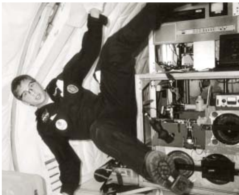
Mechanical engineering PhD student Gwenael Chiffolleau experiences zero-gravity in NASA's KC-135 astronaut-training aircraft at the Johnson Space Center in Texas. The flammability of metals in weightless, oxygen-enriched environments was tested during the visit for a research project involving our Phenomena in micro-Gravity (PiG) Laboratory and the NASA Johnson Center's White Sands Test Facility in New Mexico.
