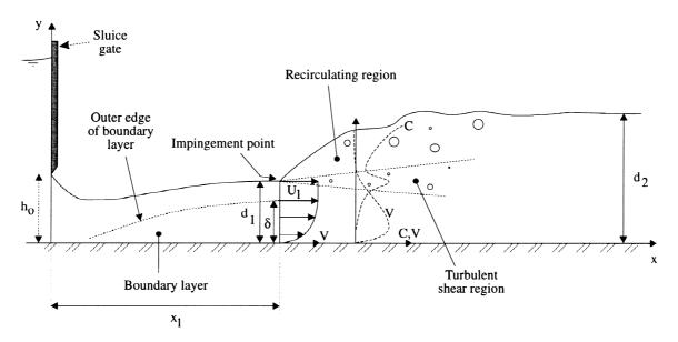
Fig. 1. Sketch of the hydraulic jump flow experiment.
