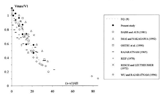
Fig. 5. Dimensionless maximum velocity  $V_{\text{max}}/V_1$ : comparison between data (Table 1) and Eq. (8).
