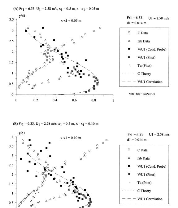
0 0.2 0.4 0.6 0.8 1 Fig. 2. Typical distributions of air concentration, dimensionless velocity and dimensionless bubble frequency (present study).
