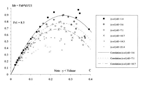
Fig. 8. Dimensionless bubble frequency ( $f_{ab} = F_{ab} \times d_1/U_1$ ) distribution in the turbulent shear region as a function of the local air content C—comparison with Eq. (15).
