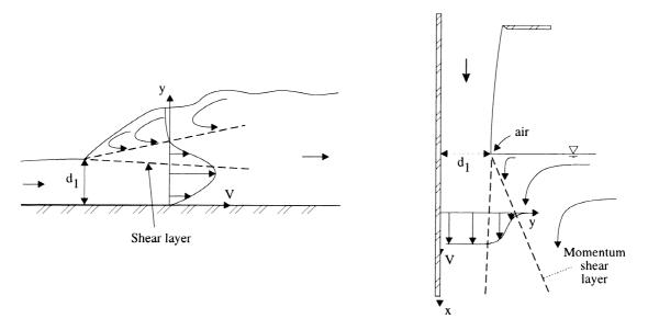
Fig. 10. Transfer of momentum and fluid entrainment process in developing shear layers at hydraulic jump and vertical plunging jet.
