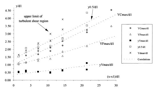
Fig. 9. Dimensionless characteristic parameters as functions of the dimensionless distance from the jump toe— Comparison with empirical correlations (Eqs. (2), (4), (9), (10) and (13)).
