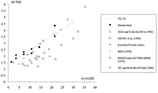
Fig. 6. Dimensionless distance  $y_{0.5}/d_1$ : comparison between data (Table 1) and Eq. (9).
