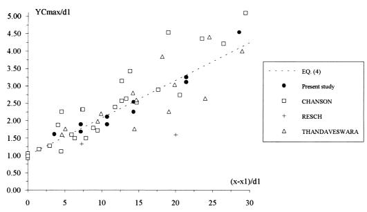
Fig. 4. Location of the maximum air content  $Y_{C_{max}}/d_1$  in hydraulic jump with partially developed inflow conditions: comparison between Eq. (4) and data (present study, Chanson, 1995a; Resch and Leutheusser, 1972, Thandaveswara, 1974).
