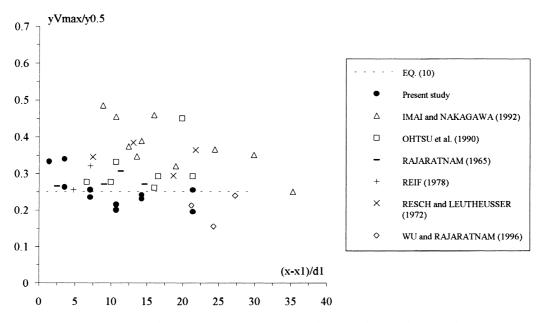
Fig. 7. Dimensionless distance  $y_{V_{max}}/y_{0.5}$ : comparison between data (Table 1) and Eq. (10).
