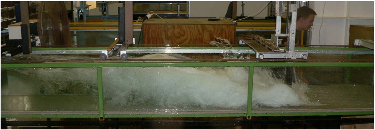
Photograph of a hydraulic jump in laboratory ( Fr_1 = 11 ) - Flow direction from right to left
